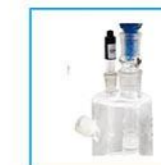
Coulometric electrolytic cup Suitable for micro moisture samples
