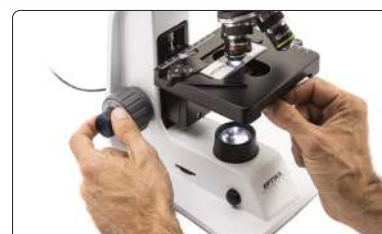
Regulation of diaphragm aperture
