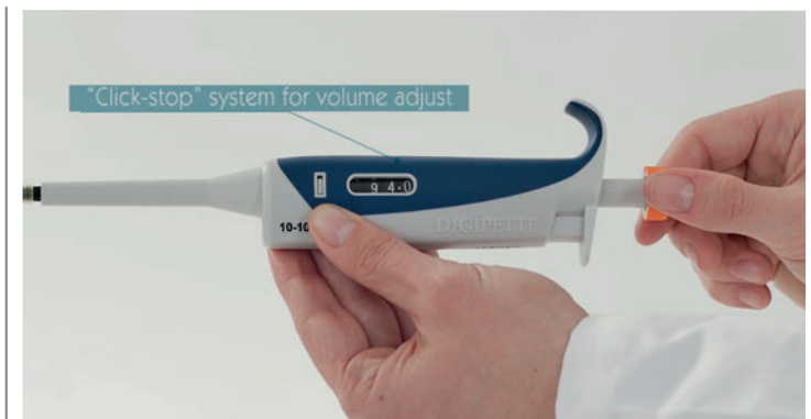
“Click-stop” mechanism of volumen selection
